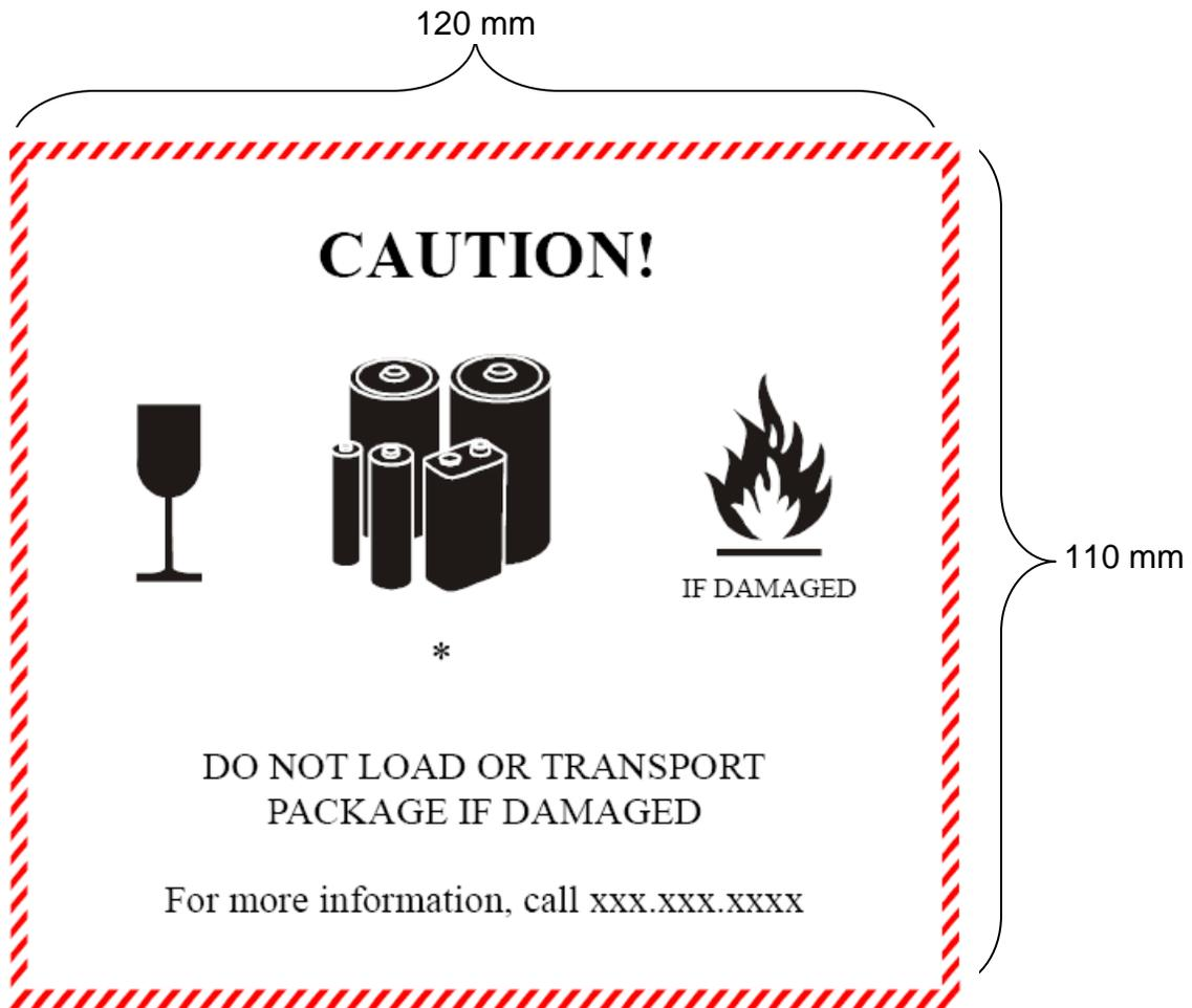
\* Place for "Lithium ion battery" and/or "Lithium metal battery"
