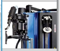
This mounting tool guides the tyre during the mounting procedure, and assisted by the bead pusher the upper bead breaker disc presses the tyre most gently into the drop centre of the rim.
