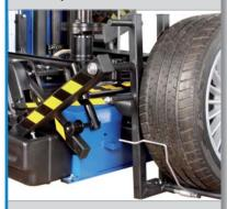
The data is used to position the clamping flange automatically and exactly relative to the wheel. Then the lift loads the wheel onto the clamping flange where the wheel is clamped hydraulically.
