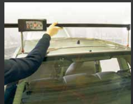
Windshields & Back Glass Any point-to-point length, width or diagonal measurements.
